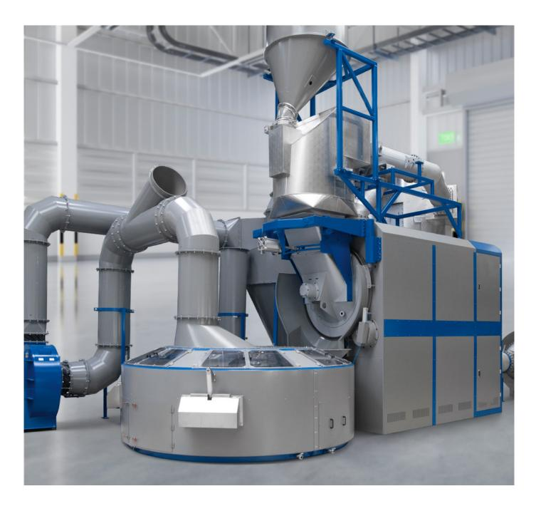
More than a drum – The MAESTRO combines traditional drum roasting with the proven properties of the RFB roasting technology. The CONDUX damper system allows the ratio of convective and conductive energy input to be variably controlled. New design solutions for energy transfer management and advanced software tools such as PROFILE DESIGNER, DARK ROAST and TRIPLE-A enable a wide range of roasting profiles that goes well beyond the conventional range.
