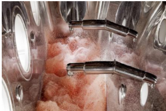
The fluidised bed provides optimum conditions for effective mass transfer and heat exchange.
