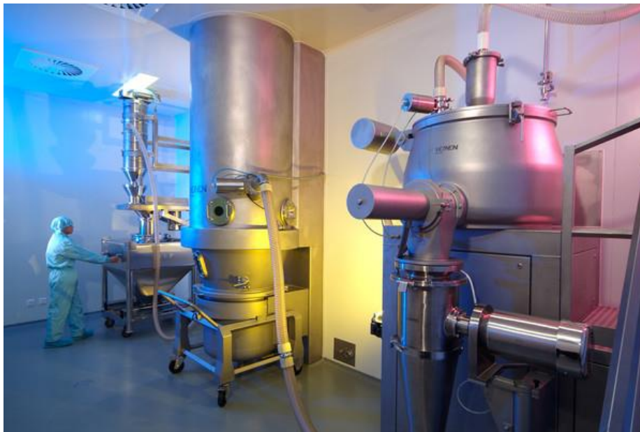
Batch processing in a Batch FB plant is particularly effective with frequent product changes.
